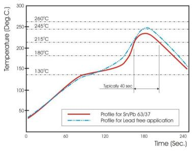
Fig 3. Infrared soldering profile for Chip Resistors WW12
