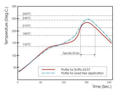
Fig 3. Infrared soldering profile for Chip Resistors WW25T
