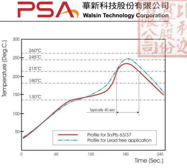
Fig 3. Infrared soldering profile for chip resistor
