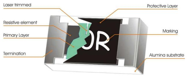
Fig 1. Construction of Chip-R
