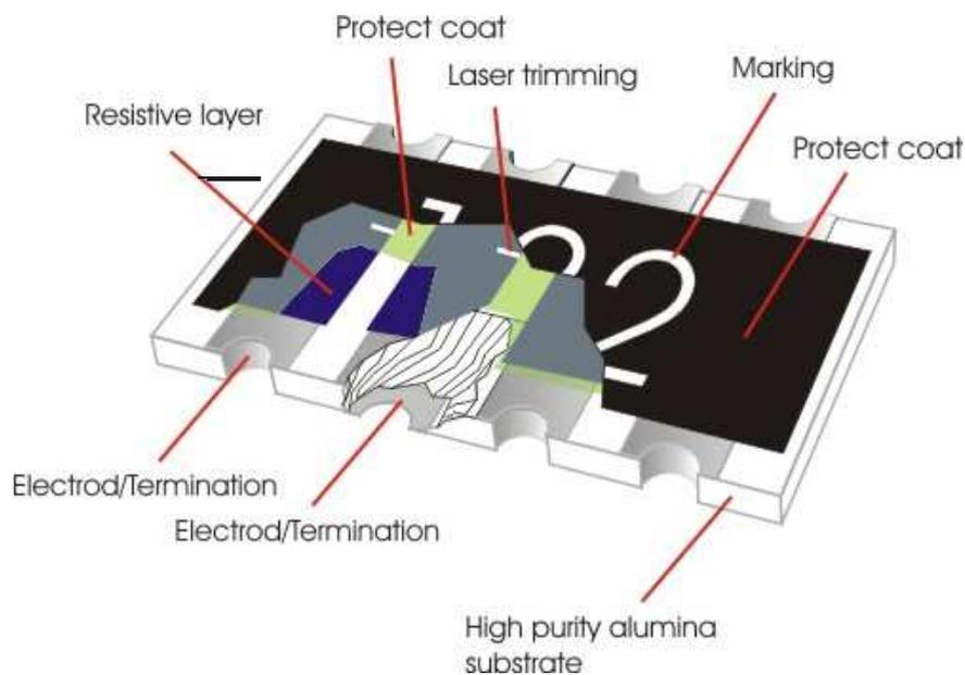
Fig 1. Construction of a Chip-R array WA04T
