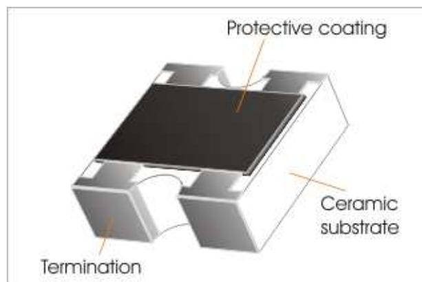
Fig 1. Construction of a Chip-R array WA06Y
