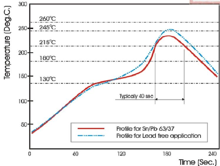
Fig 3. Infrared soldering profile for Chip Resistors array
