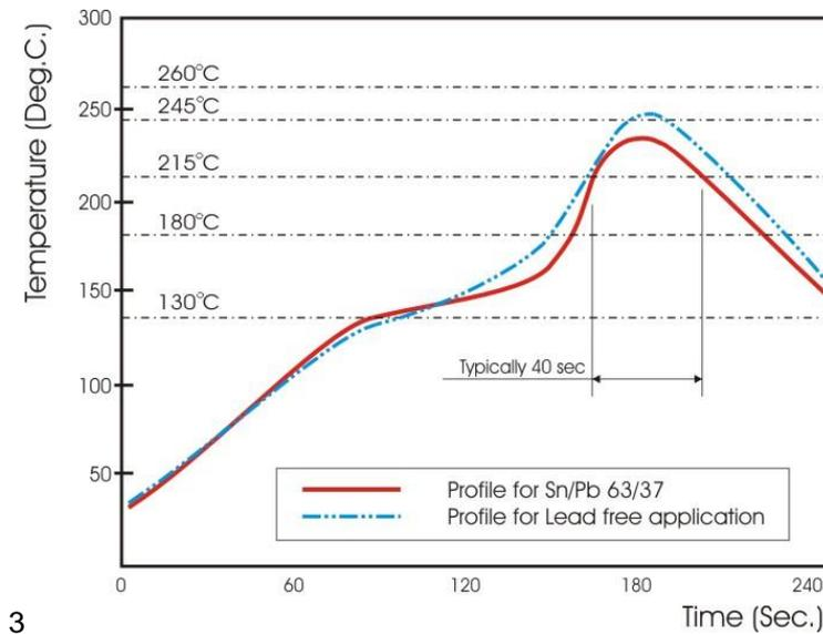
Fig 3. Infrared soldering profile for Chip Resistors WW25Q
