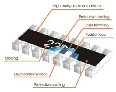
Fig 1. Construction of a Chip-R array WA06W\_N
