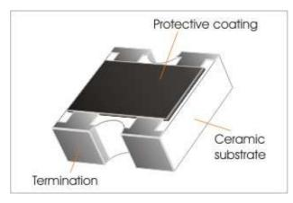
Fig 1. Consctruction of a Chip-R array WA06Y
