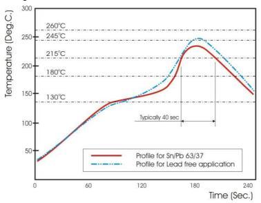
Fig 3. Infrared soldering profile for Chip Resistors WW25
